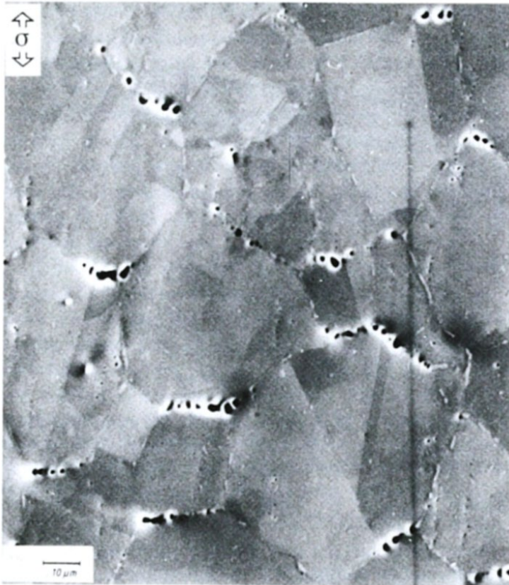
316 SS pre-implanted to 100 appm He and creep tested at 1023 K – preferred bubble growth on GBs perpendicular to applied stress
