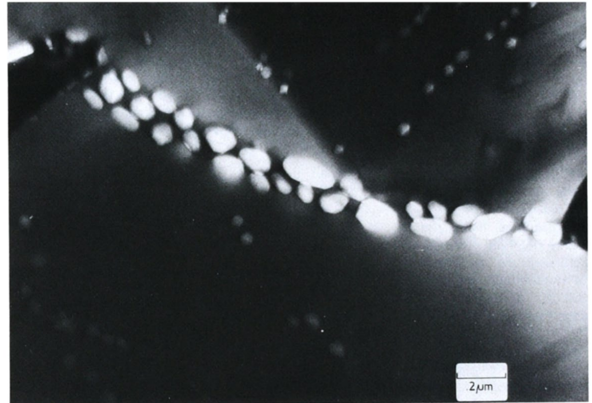
316 SS tested at 1023 K for 25 hr at a stress of 50 Mpa and a final He concentration of 2500 appm
